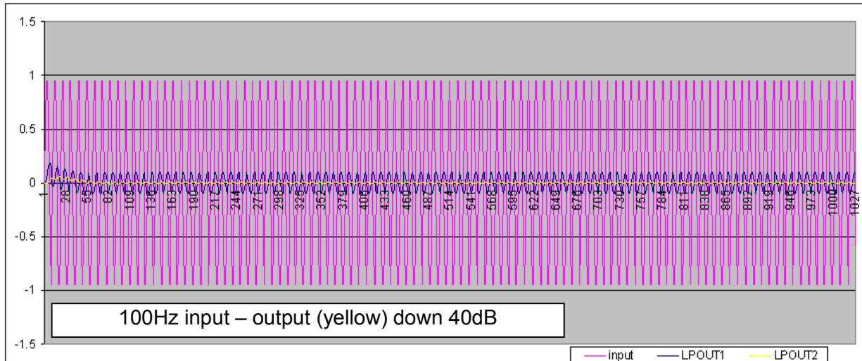
The previous 7 graphs showed a 2<sup>nd</sup> order 10Hz LP filter with  $\zeta = 0.71$ . At low frequencies, there is little output attenuation (yellow trace) but as the signal approaches 10Hz there is an attenuation of about 3dB and this becomes 40dB at 100Hz i.e. 40dB per decade as expected. At 50Hz the output is down 28dB i.e. 12dB higher than 100Hz.
